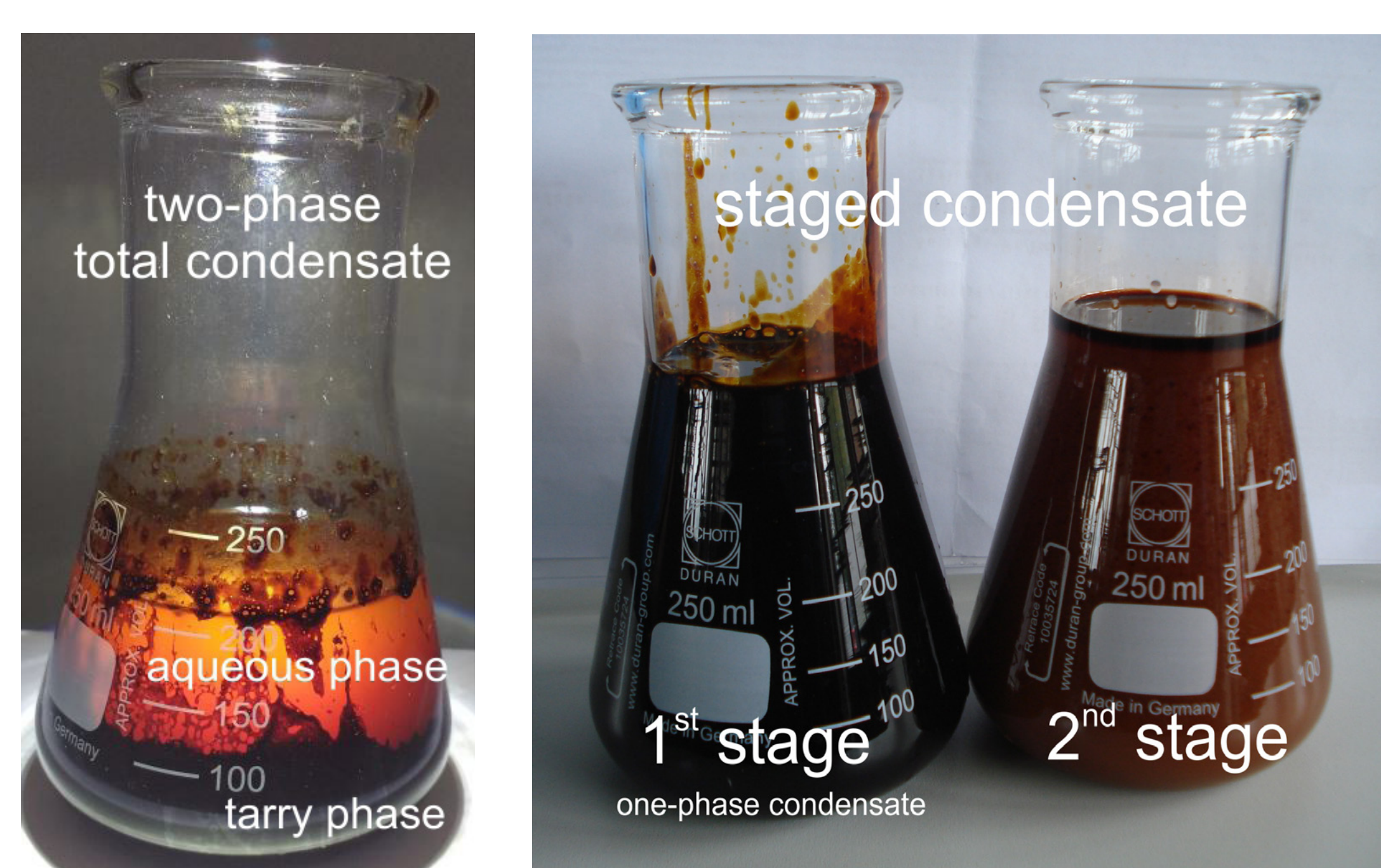
Fig. 1: Two-phase total condensate (left) and single-phase staged condensate (right).
