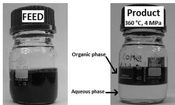
Figure 1: Feed and product of hydrotreatment at 360 °C and 4 MPa
