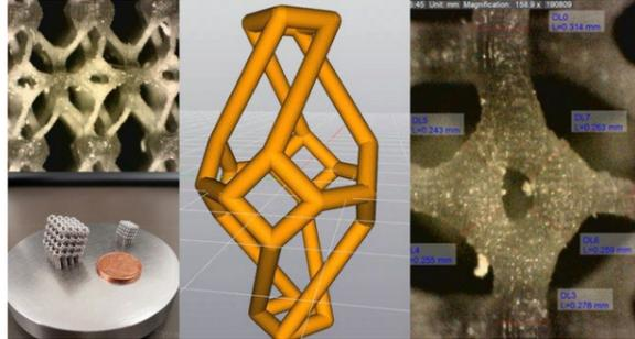
The AERIALIST project disclosed the potential of metamaterials in aeronautics through four pillar actions: i) consolidated the aeroacoustic theory of metamaterials; ii) developed and assessed methods for efficient additive manufacturing of metamaterials; iii) validated models and design through wind-tunnel experiments; iv) assessed the entire toolchain loop modelling-manufacturing-experiments and provided a development roadmap towards TRL of industrial relevance.
